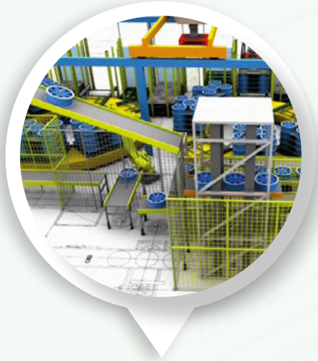
Photo: Simulation model of a tire mounting, sorting and buffering system
