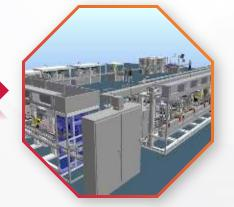
Mechanical & Logic operations validated prior to site. Reduced time between design complete and production milestones.
