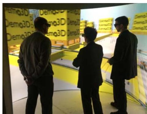
The users can move freely in the simulation model and have a 250° panoramic view, which facilitates the mental immersion into the system. In the prototype, up to six people fit into the CAVE at the same time. However, the concept could be extended to allow for more users.
