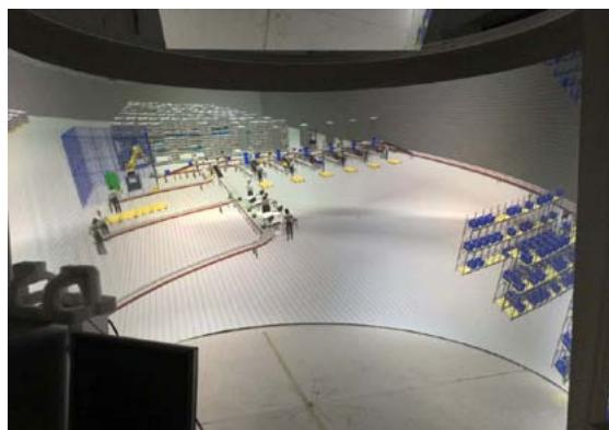
The research project „VIFA3D – Virtuelle Fabrikplanung in der 3D-CAVE“ (VIFA3D - Virtual Factory Planning in the 3D-CAVE) developed a solution that can support the planning process. The project combined the concept of virtualisation in the 3D-CAVE with material flow simulation in production and logistics systems and thereby created a planning and communication tool.
