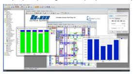
At the preliminary phase of the project, material flow simulation was used to support the early planning phases of painting plants for vehicle fixtures. For this, the current planning stage was modeled in order to be able to recognize any weaknesses early on and to modify the layout accordingly. Since the software Plant Simu-
