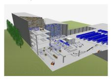
Klug also uses project-specific Demo3d videos for customer communication. This way, the planned automation technology and logistics processes can be presented tangibly already during the sales and project planning phase. In contrast to static CAD-drawings and excel spreadsheets, this facilitates comprehension of the proposed concept.
